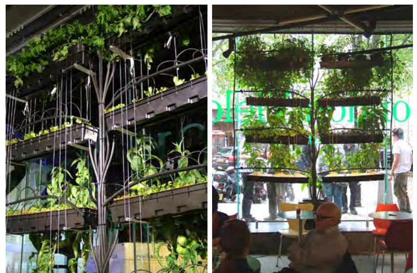
Fig.8: The Urban Agriculture Curtain. A working prototype for a vertical productive urban landscape as part of the exhibition “London Yields”. The system developed with Hadlow College utilizes industry standard hydroponics components and produces fortnightly crops for use in the Building Centre’s restaurant. Image: Bohn&Viljoen Architects, 2009
